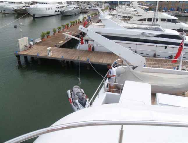
Lowering PWC to Main Deck Level
