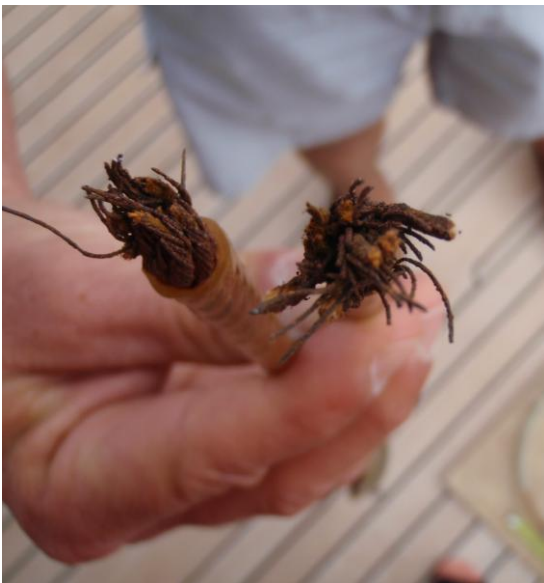
Close up of sling failure
