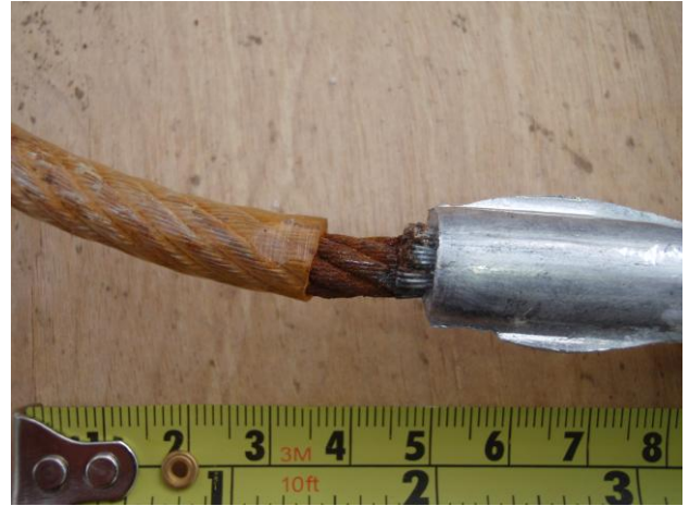
Metal Swage on Sling from Recovered Harness (Soft Tape removed)
